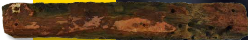
1. Beam before (a) and after (b) mechanical cleaning/ Greda prije (a) i nakon (b) mehaničkog čišćenja (Photo: M. Šimičić, M. Bačić)
